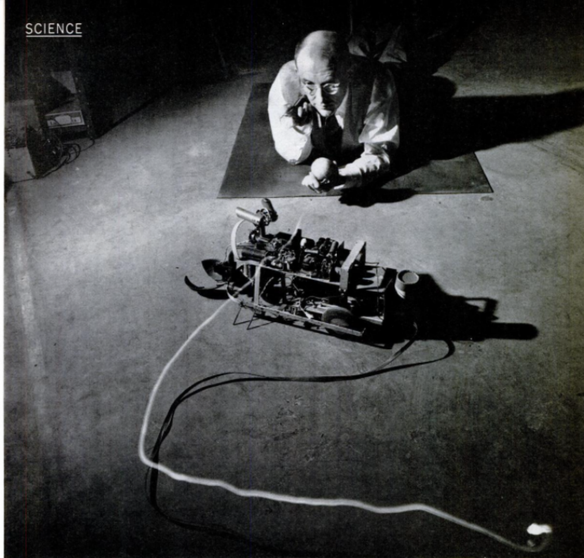
BERKELEY BECKONS "SQUEE" WITH FLASHLIGHT WHOSE BEAM, STRIKING PHOTOCELLS MOUNTED IN TUBES ON TOP, MAKES IT "FIND" AND PICK UP BALL
