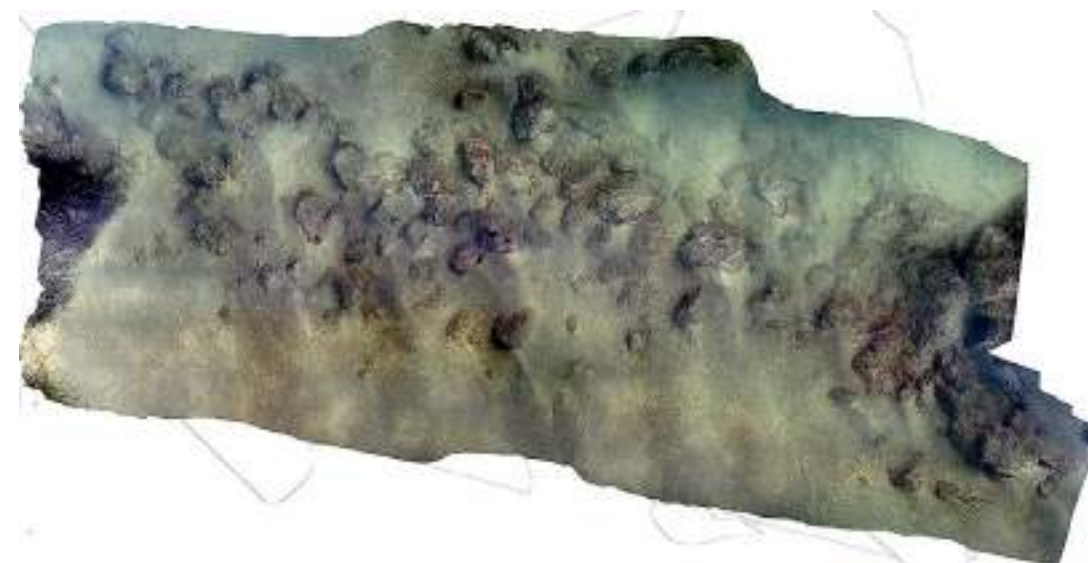
Fig. 2. Orthophoto created out of a 3D-model made by Agisoft Photoscan using action cam screen shots. Meninx project. 2017. Orthophoto: M. Fiederling
