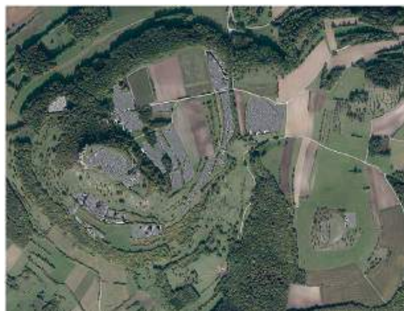
Fig. 2. Staffelberg. Satellite image of the Bayerische Vermessungsverwaltung fused by magnetometer measurements from 1987–2017. Magnetogram: J. W. E. Faßbinder, F. Becker
