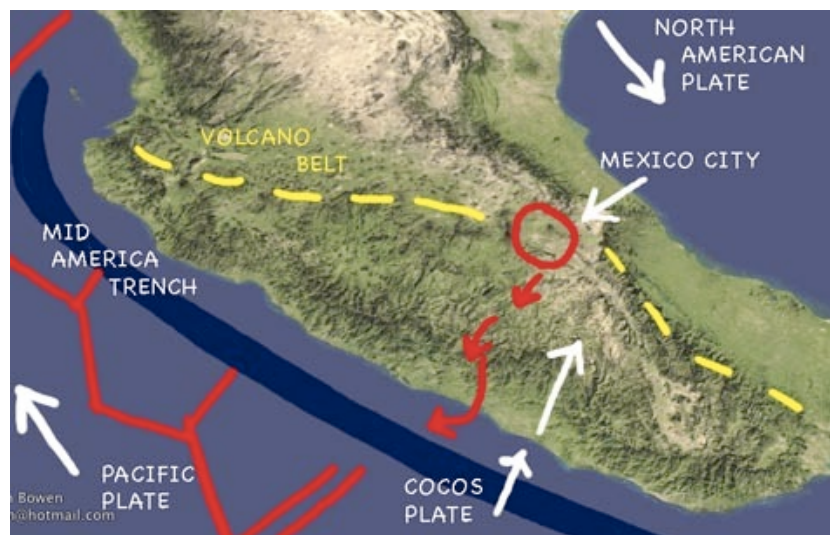
Figure 14. Interaction of Tectonic Plates that Caused the 19 and 21 September 1985 quakes in Mexico
