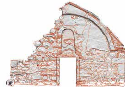
Fig. 8: a – West façade drawn from hand measurements; b – Line drawing of the west façade of St. Petka's (red) superimposed on the point cloud
