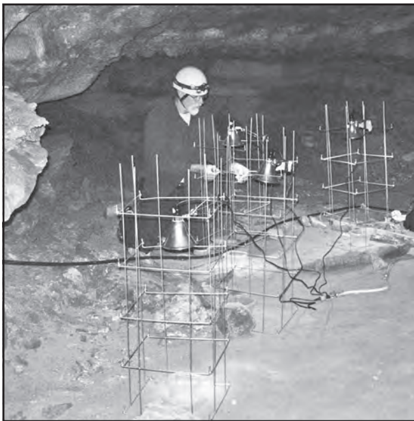
Figure 3: Mammoth Cave ecologist, Rick Olson, sets up an experimental apparatus to measure the amount of algae growth that occurs under different lighting conditions. MCICSL is co-lead on this project, which is also taking place at four other national parks.
