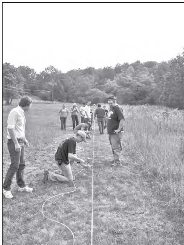
Figure 1: Wittenberg University geology students use Electrical Resistivity Ground Imaging to look for cave passages near Mammoth Cave National Park. MCICSL staff helped coordinate the activity.
